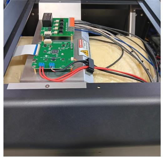
3. Find the USB-C port on the Blue Alpine data PCB (the green board on the right side of the machine) and plug in the USB-C connector.
