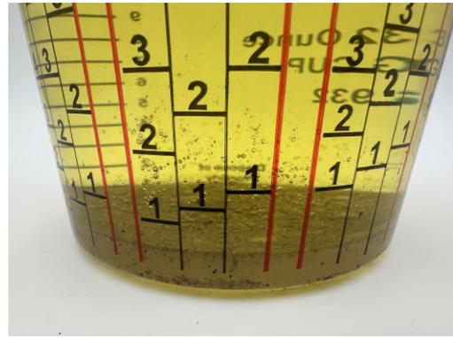
**Note:** Used oil will often have black particles in it, this is material from the casting of the pump and is normal.
