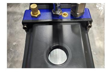
7. After your first batch, the break-in oil should be replaced. See vacuum pump maintenance on page 30 for oil change instructions.
