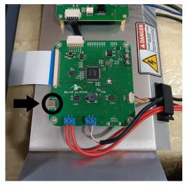
5. Press the reset button twice\* to activate download mode. The GCM4BOOT drive window should pop up on your computer and will act like a USB drive; if not, check the connected USB devices on your computer and see if this drive is found.
