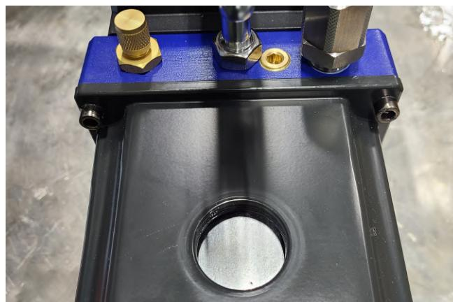
Setup for a commercial pump is virtually the same as the premium pump except the use of KF fittings instead of threaded fittings. It is important for the commercial pump to set the gas ballast valve to open. See the diagram for how to install a KF fitting, or the video below.
