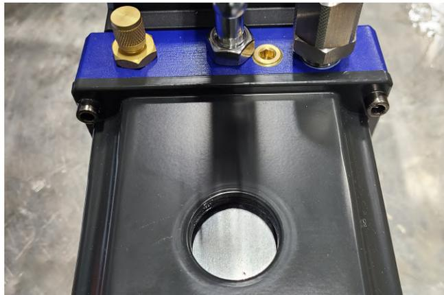
6. Reattach the oil mist filter. **Note:** On the premium pump, the threads on the oil mist filter are plastic and can break if tightened too hard. For best results, tighten only until snug.
