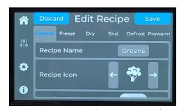
**Note:** Preset recipes can only be edited while a batch isn't running. To edit a recipe select **Recipes** from the home screen. Select the recipe you would like to edit. Press **Edit** Adjust settings in each tab as needed, then press **Save** in the upper right corner.
